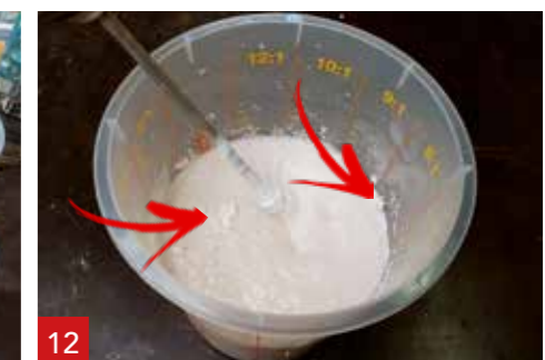
12 Stir the mixer till all lumps have disappeared (± 1 min.) resulting in a smooth material.
