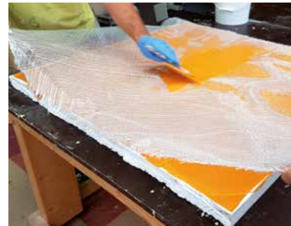
Before applying the A1 Triaxial fibre, cut it to size first, given the processing time of A1.
