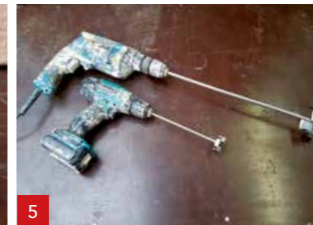
5 Choose the appropriate mixing machine.
