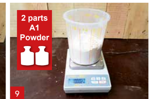
9 Weigh 2 parts of A1 Powder. In this example we use 1000 g A1 Powder.
