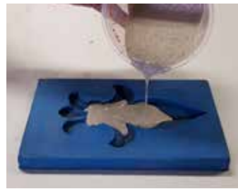
Pour part of the created A1 into the mould. Start (if possible) by brushing the mould, so that all unevenness/relief is touched with A1.
