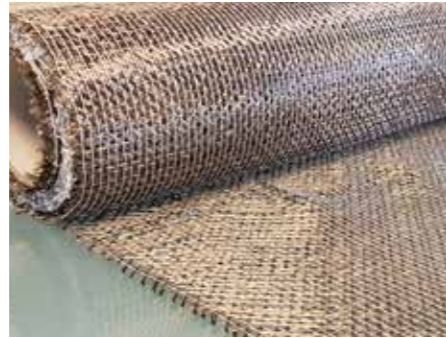
A1 Triaxial basalt fibre 160 gr/m 2
