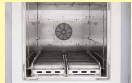
Roller conveyor in furnace chamber
