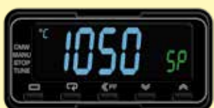
Example of an over-temperature limiter
