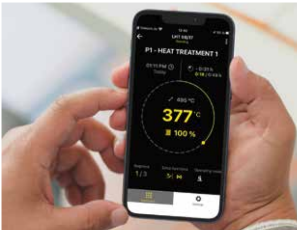
Display of program progress for each furnace
