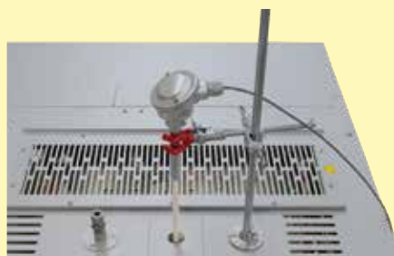
Thermocouple port in the ceiling with tripod
