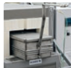
Hardening boxes with protective gas connection
